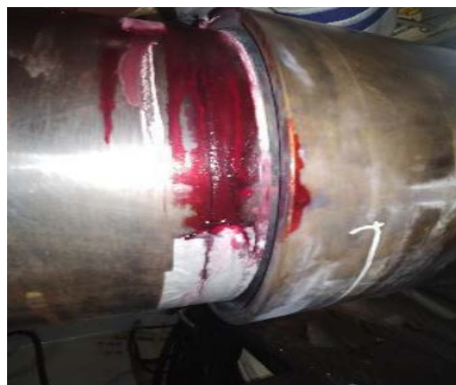
Figure 2 Recent example of cracking that required replacement of the propeller shaft
